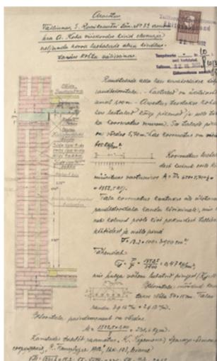
**Figure 26.** Calculations of the wall strength of the building at 8b *Roosikrantsi* Street, Tallinn (1932).
